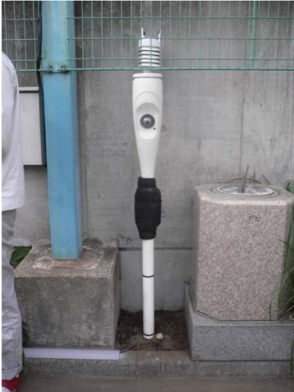
An almost front on view of a field server manufactured by Matsushita Electric Works Server is equipped with a rubber cover to ensure the safety of the Visala sensor attachment
